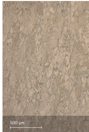
Microstructure solution annealed Etched with etchant Kallings 2
