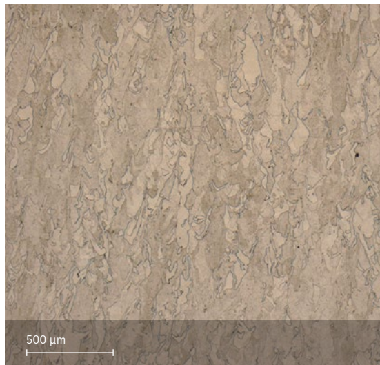
Microstructure solution annealed Etched with etchant Kallings 2
