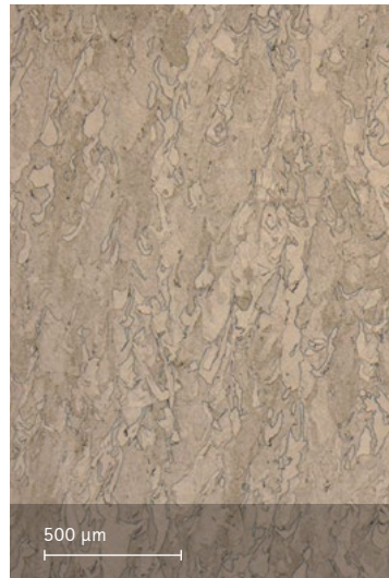
Microstructure solution annealed Etched with etchant Kallings 2
